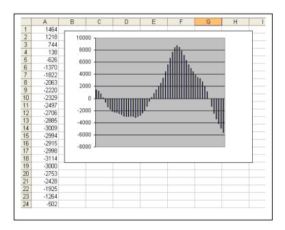
PCM data – which is how sound is encoded on CDs - uses numbers in the range of +32767 to -32768, <sup>18</sup> and takes a sample every 1/44100<sup>th</sup> of a second. (for audio CDs)
