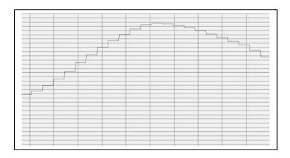
Above shows that the smooth waves are in fact made of discrete steps. Each step represents 1/44100 of a second.
